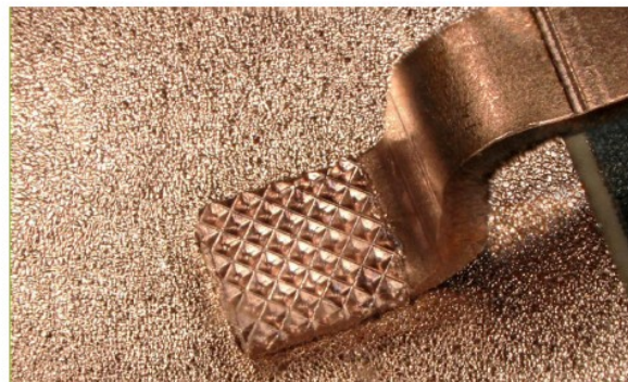
Figure 2 Smart Welded Terminal Smart Welded Terminal on Direct Bonded Copper (DBC – ceramic isolation between thick copper layers)
