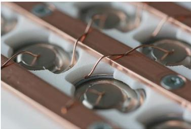
Figure 9: Detail of battery pack produced with copper wire
