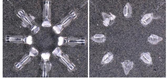
Figure 3: Al bonds and their shear test residues on a battery cap of nickel-coated steel, made at room temperature with parameter set 1 (length 520 ms)
