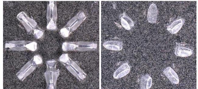
Figure 4: Al bonds and their shear test residues on a battery cap of nickel-coated steel, made with shortened parameter set 1 (length 150 ms) with the bonding tool at 430 $^{\circ}$
