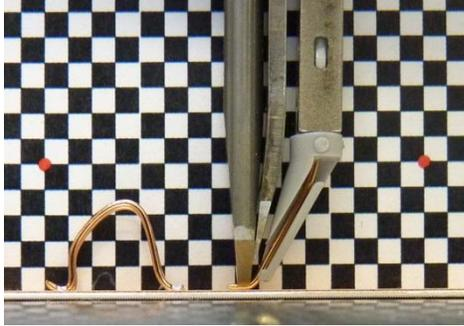
Fig. 1: Copper wires bonded onto a copper substrate
