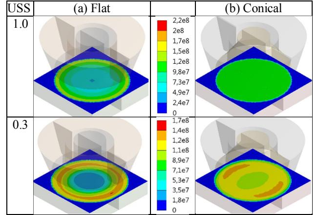
**Fig. 8: Pressure distribution between pin and substrate for different ultrasonic softening states of the pin in case of flat (a) and conical (b) tool shape**
