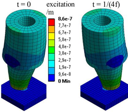
**Fig. 3: Pre-stressed vibration system with oscillating forces  $F_x$  and  $F_z$**
