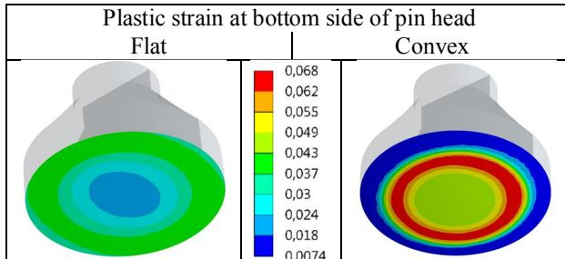
**Fig. 7: Plastic strain at bottom side of pin head in case of flat and convex shape**
