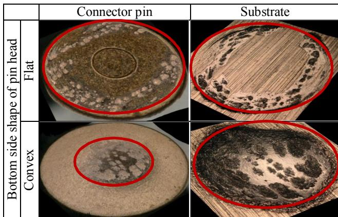
**Fig. 12: Shear surface of connector pin and substrate for flat and convex pin design**
