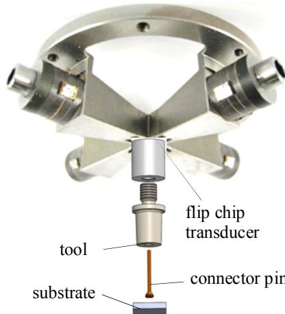
**Fig. 2: Exploded view of multidimensional vibration system**
