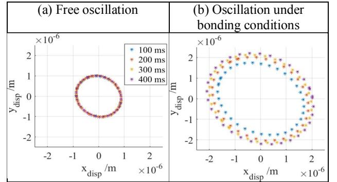
**Fig. 10: Vibration amplitude in bonding plane at tool tip in case of (a) free oscillation and (b) bonding**
