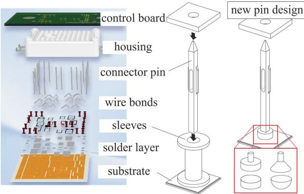
**Fig. 1: Assembly of a power module with pressfit contact between connector pin and control board using the current pin/sleeve compound and conceivable designs of the connector pin for ultrasonic bonding**
