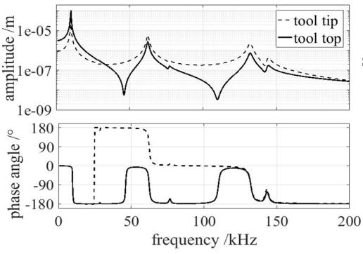
**Fig. 4: Frequency response at topside of the tool as well as tool tip**
