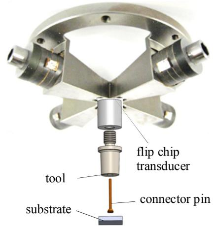
**Fig. 2: Exploded view of multidimensional vibration system**
