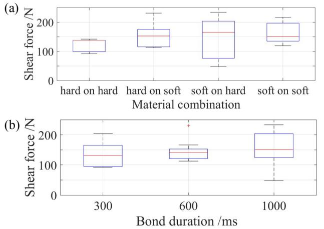
**Fig. 11: Shear force for different (a) material hardness combination (b) bond duration**
