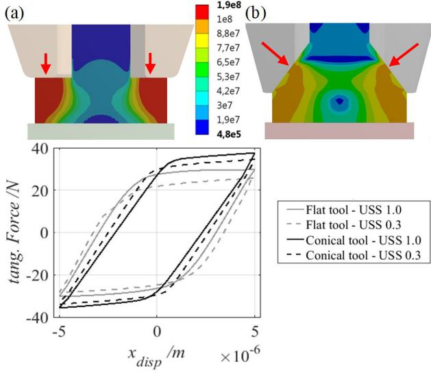
**Fig. 6: Von-Mises stress and tangential force-displacement diagram for different softening states of the pin in case of flat (a) and conical (b) tool shape**
