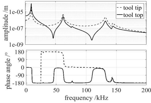
**Fig. 4: Frequency response at topside of the tool as well as tool tip**
