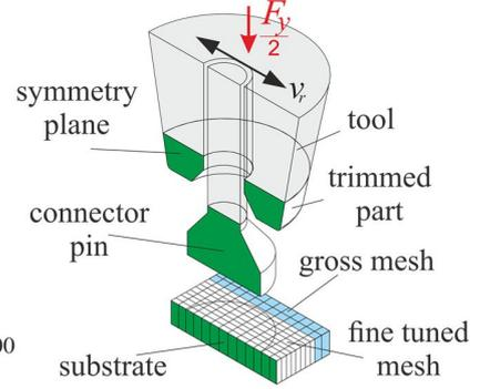
**Fig. 5: FE model of ultrasonic bonding of connector pin**
