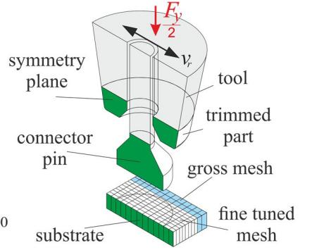
**Fig. 5: FE model of ultrasonic bonding of connector pin**
