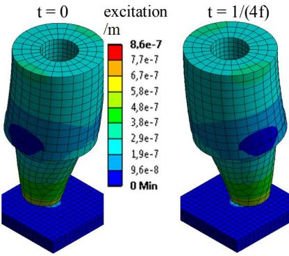
**Fig. 3: Pre-stressed vibration system with oscillating forces  $F_x$  and  $F_z$**
